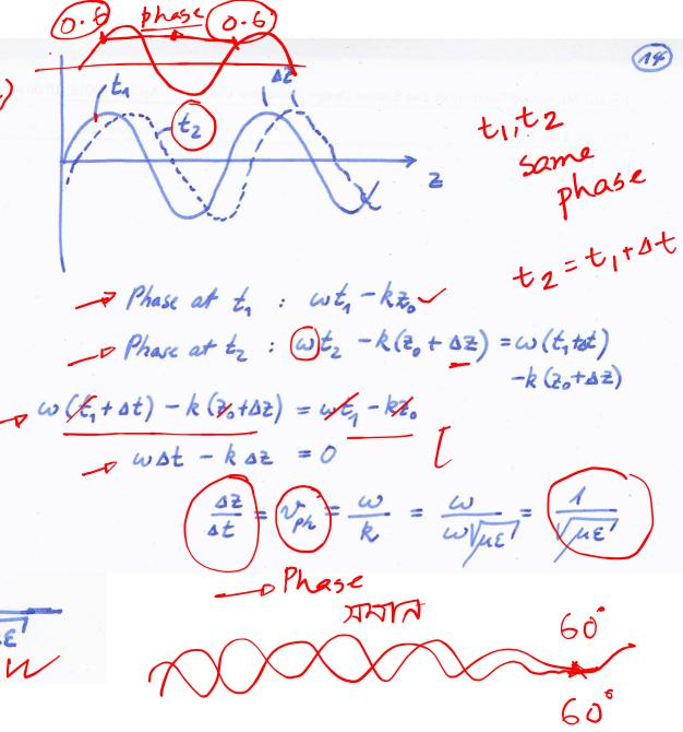
A plane wave propagates in a lossless medium. The electric vector field is given as:
